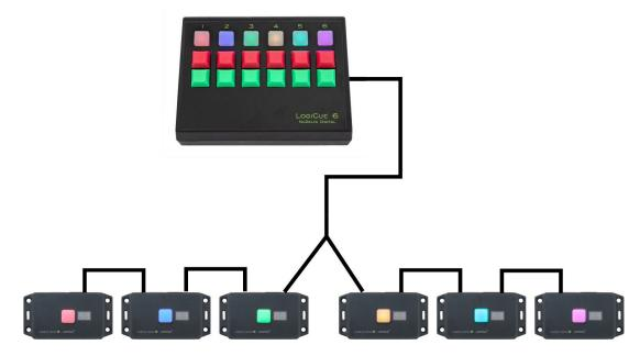
The LogiCue System is designed to be connected together with standard microphone cable. Not all microphone cables meet our standards. We have found low cost microphone cable that when analyzed, only had one single strand of copper carrying the signal in some spots. While this type of cable may carry an audio signal a short distance, the LogiCue signal requires enough current to power the cue lights and therefore may not work with poor quality cable.
