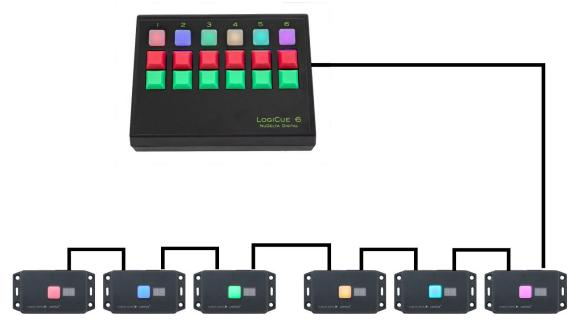
The signal for the LogiCue System can also be split using "Y" cables or other passive splitting devices (not included). The signal cannot go through transformer isolated splitters or digital audio snakes.
